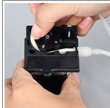
Step 3 Install the pump hose
